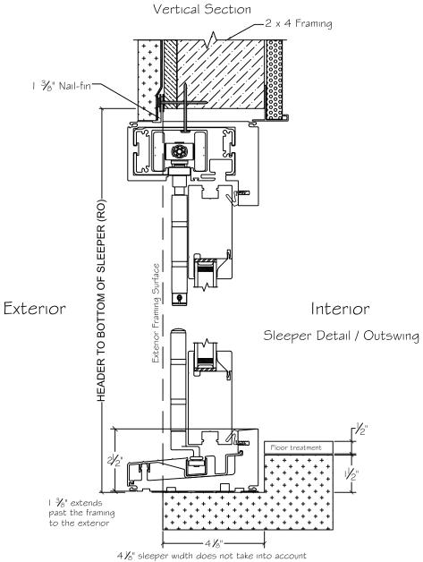
$4\,\mbox{1}_8"$  sleeper width does not take into account pans, membranes  ${\bf \hat{t}}$  sealant provided by others.
