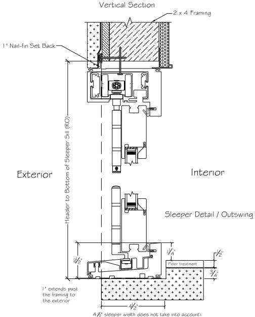
$4\,\mbox{\ensuremath{\mbox{\it N}}}{}_2$  sleeper width does not take into account: pans, membranes  $\mbox{\ensuremath{\mbox{\it $\$}}}$  sealant provided by others.
