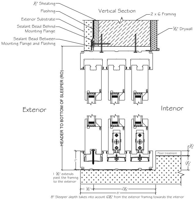
8" Sleeper depth takes into acount 6%" from the exterior framing towards the interior and 1%" extending past the exterior framing. The 1%" extension is needed to support the outer track. 8" sleeper width does not take into account: pans, membranes \$ sealant provided by others.
