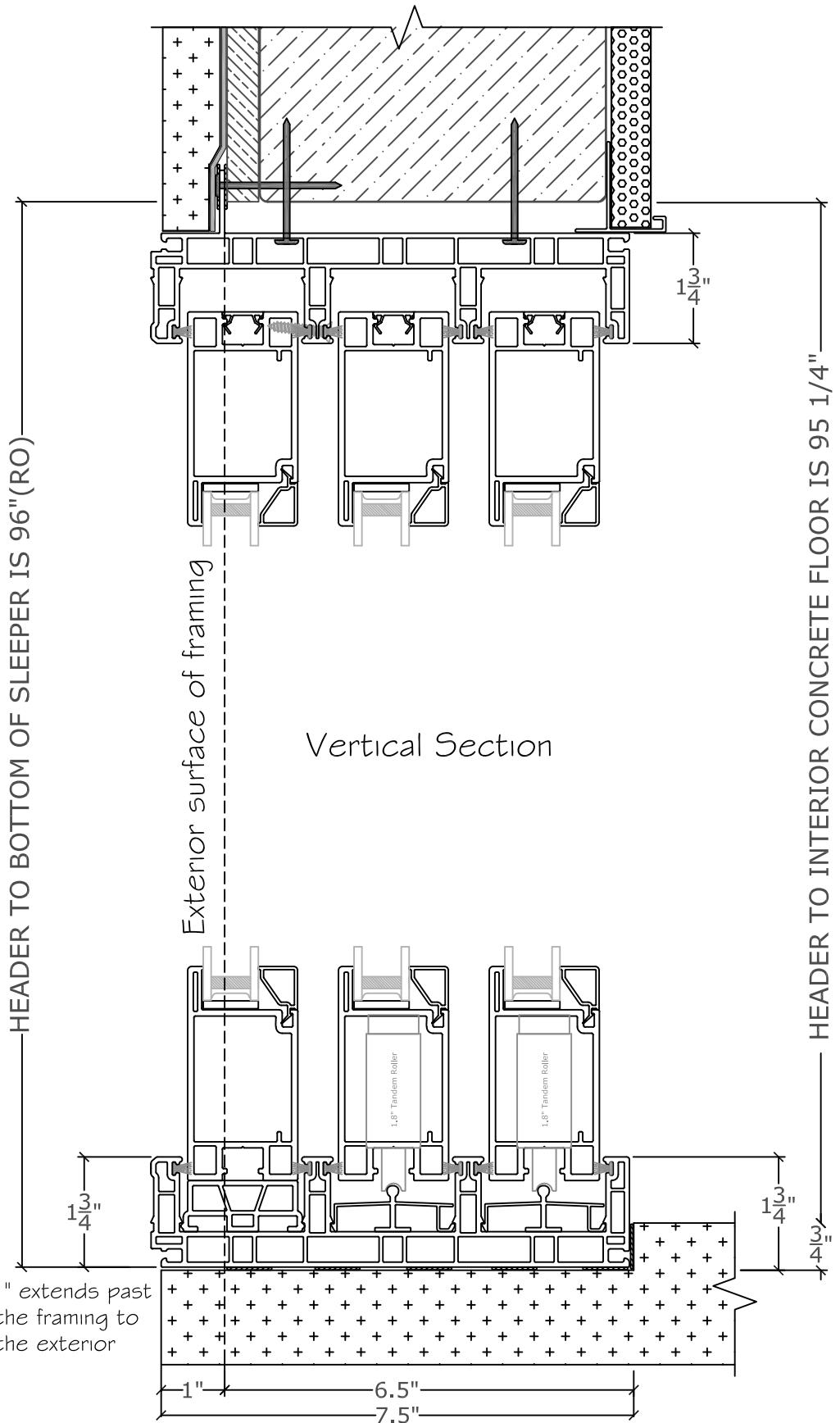
7.5" Sleeper depth takes into account 6.5" from the exterior framing towards the interior and 1" extending past the exterior framing. The 1" extension is needed to support the outer track. 7.5" sleeper width does not take into account: pans, membranes & sealant provided by others.
